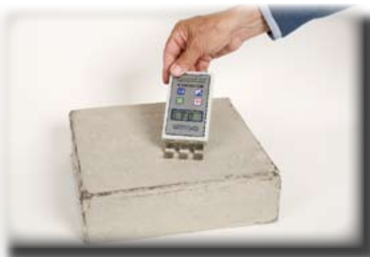
Scanning Depth 100 mm - Scans the complete Concrete slab.
