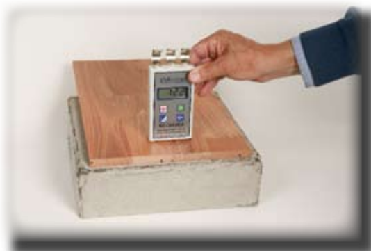
Scanning Depth 10 mm - Measures only the Wooden Floor
